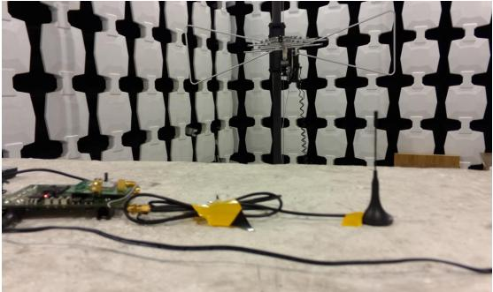
Radiated Spurious Measurement (Above 1GHz), EIRP Test Setup
