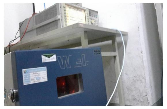
Radiated Spurious Measurement(below 30MHz) Setup
