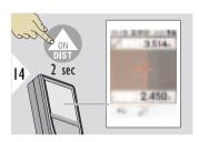
If chosen permanent measurement for second target point, the current distances are displayed.
