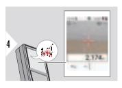
Aim laser at upper points and angle/height tracking starts automatically.
