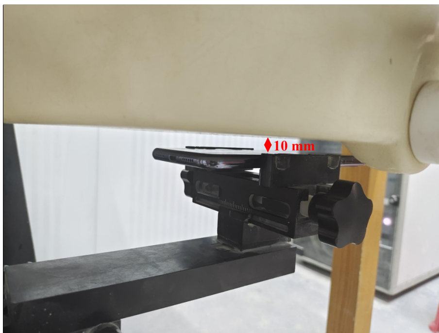
Body (Worn) Back Setup Photo (10mm)
