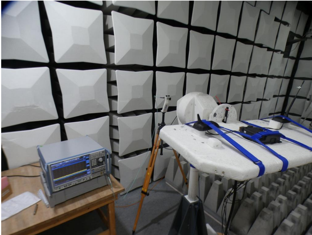
Photo 5: Test setup for radiated measurements, detailed view (above 1 GHz; Fully anechoic chamber, FCC Part 15.407; ANSI C63.10)
