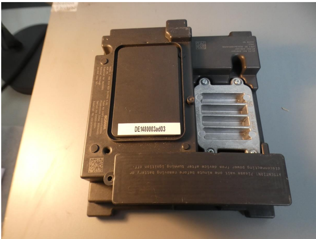
Photo 8: EUT_AD03 for conducted and radiated measurements.
