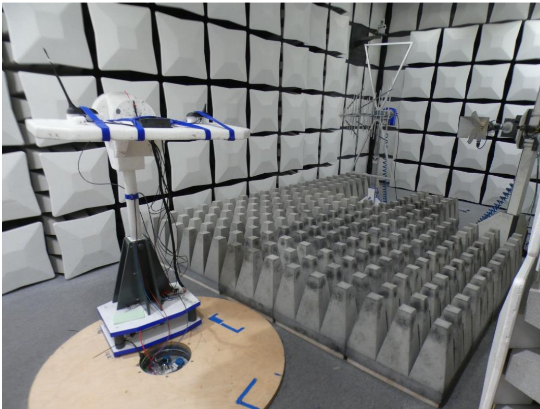
Photo 3: Test setup for radiated measurements (above 1 GHz; Fully anechoic chamber FCC Part 15.247, 15.407, 22, 24, 27 and 90; ANSI C63.10)
