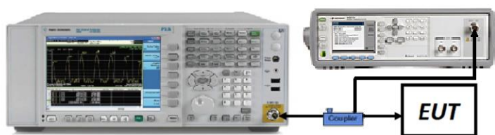
Figure 7-2. Test Instrument & Measurement Setup
