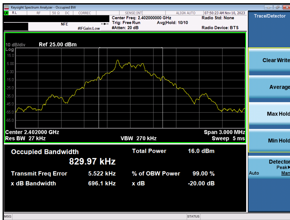
Plot 7-1. 20dB Bandwidth Plot (Bluetooth, 1Mbps – Ch. 0)
