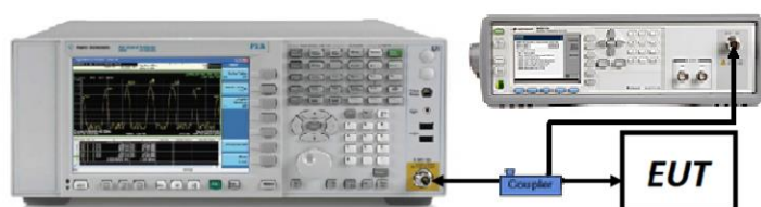
Figure 7-1. Test Instrument & Measurement Setup
