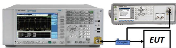
Figure 7-7. Test Instrument & Measurement Setup
