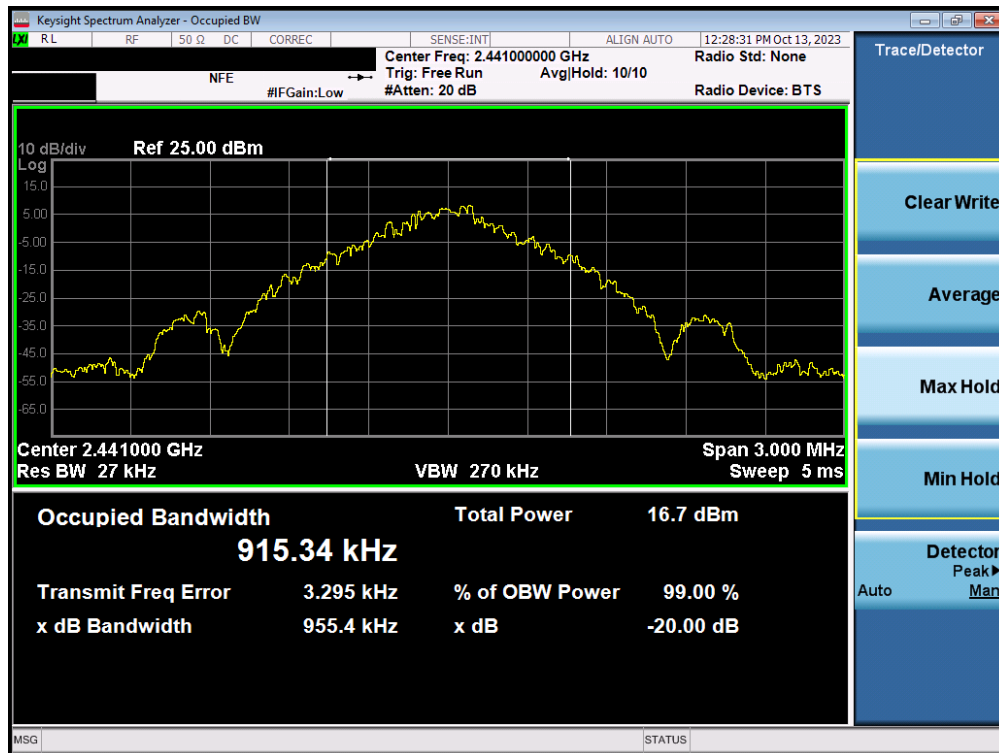
Plot 7-2. 20dB Bandwidth Plot (Bluetooth, 1Mbps – Ch. 39)
