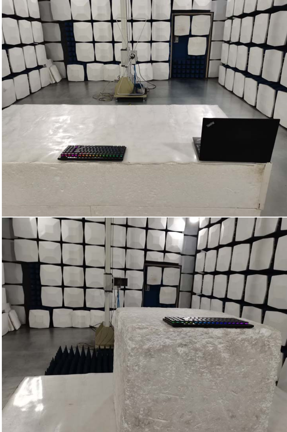
Radiated emission test view
