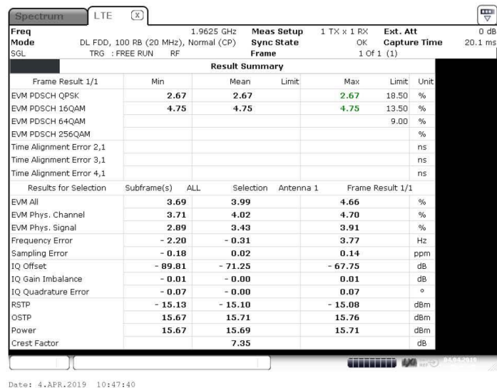
Figure 6 I/Q constellation table with I/Q error – 16QAM (1962.5 MHz) (20MHz Channel BW)
