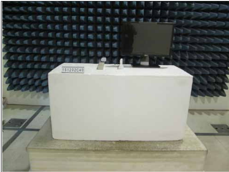
Radiated Emission Test above 1GHz
