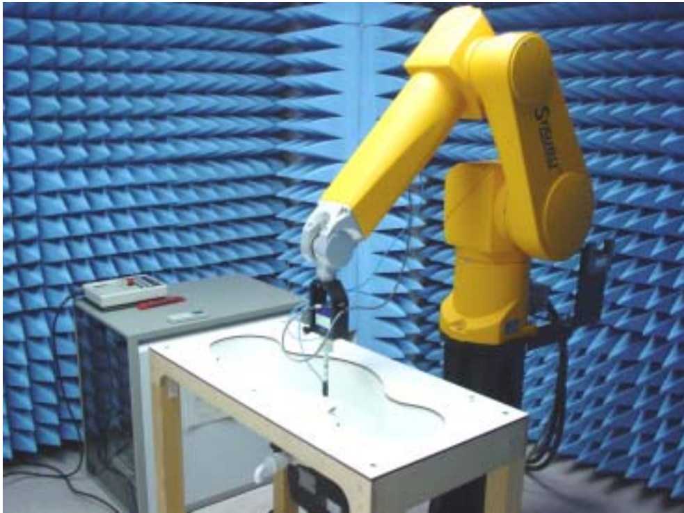
Fig.1 Photograph of the SAR measurement System
