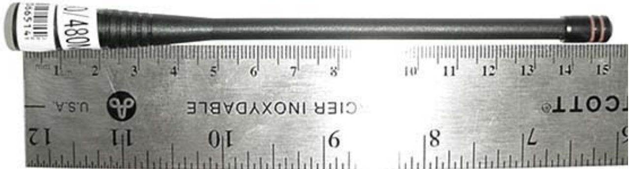
Whip Antenna (P/N: ATU-6D)
