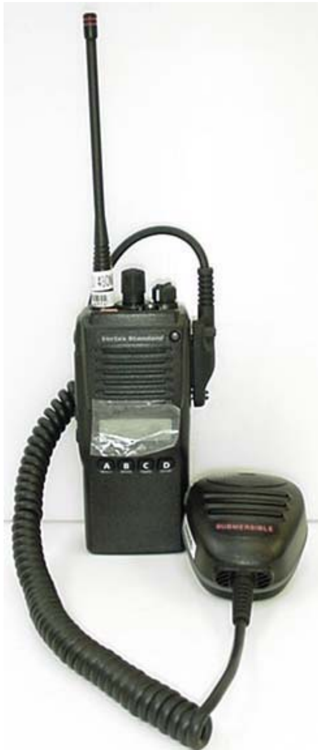
DUT with Speaker-Microphone Accessory (P/N: MH-65B7A)
