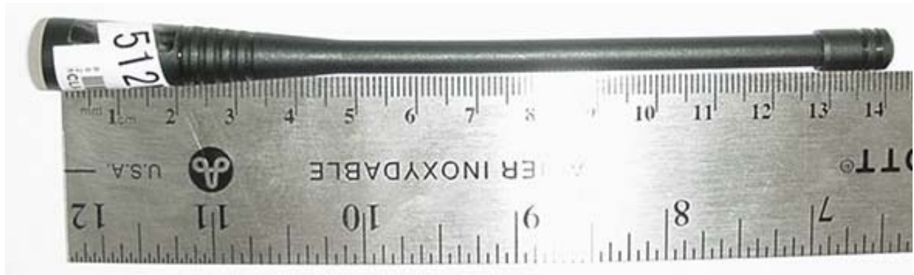
Whip Antenna (P/N: ATU-6F)
