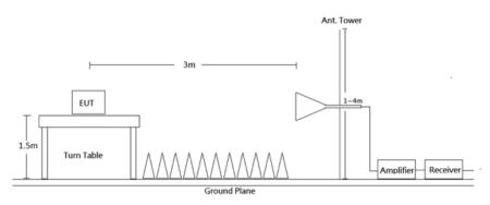
Radiated emission tests were performed in the 3 meters chamber test site, using the setup accordance with the ANSI C63.10-2013. The specification used was the FCC Part 15.209 and FCC 15.247 Limits.
