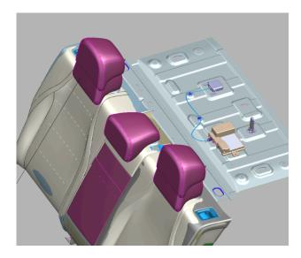
The distance to human body of internal and external antenna is more than 20cm.
