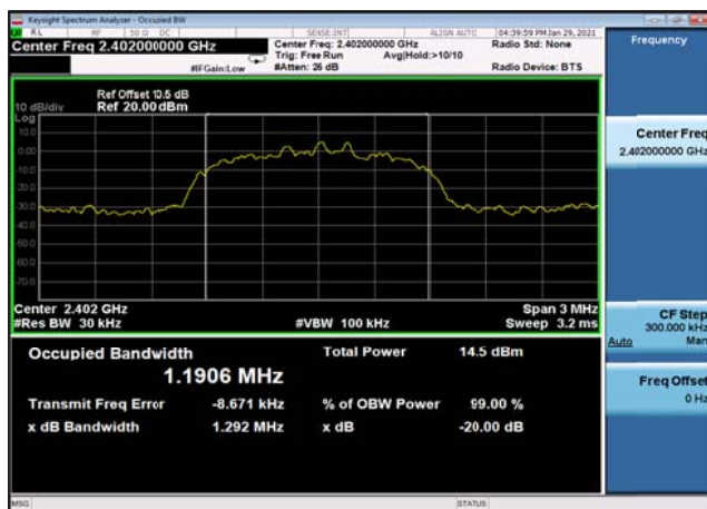
20dB Bandwidth: 8DPSK,2480MHz,3DH5
