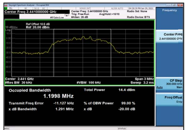
20dB Bandwidth: 8DPSK,2441MHz,3DH5
