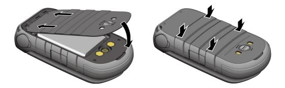
**Warning:** Press all around the edges of the battery cover ensuring it is properly sealed to maintain the phone's waterproof capability.
