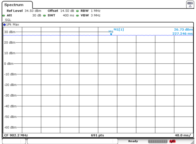
FHSS_SF10 time-domain plot duty cycle as 100%
