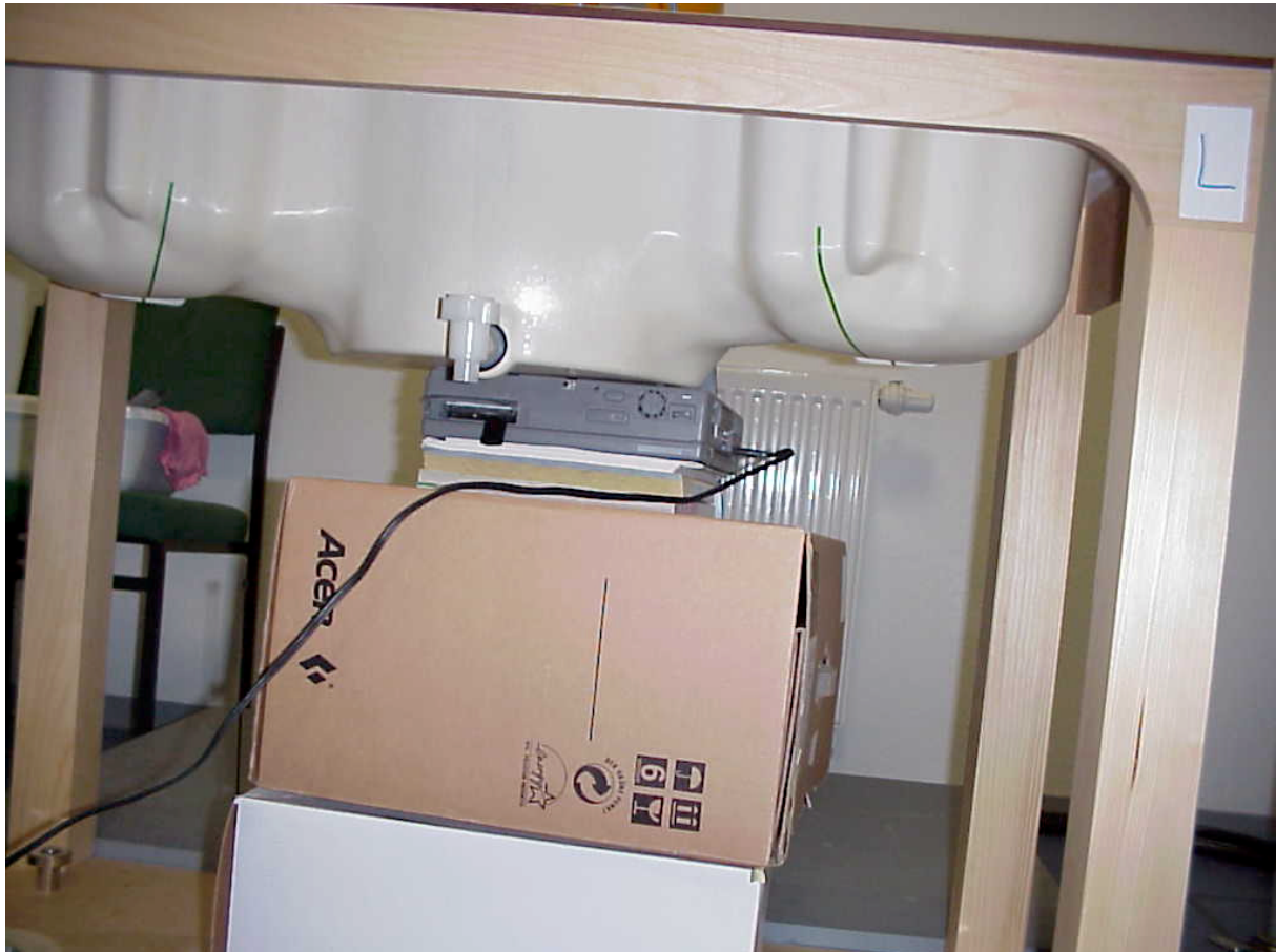
Photo 4: Position bottom on the flat phantom (Body SAR measurement)
