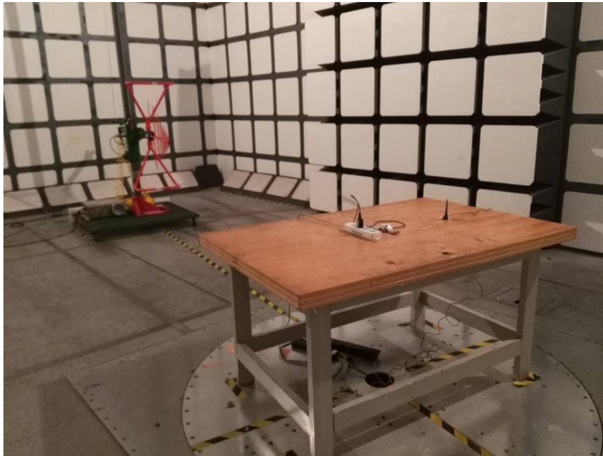
Radiated Emissions View (Above 1 GHz)
