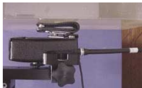
Body-worn SAR Test Setup 4.5cm Belt-Loop, Swivel, & Case Separation
