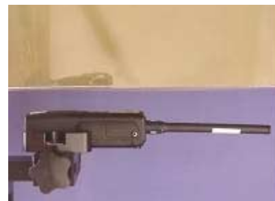
Face-held SAR Test Setup 2.5cm Separation Distance
