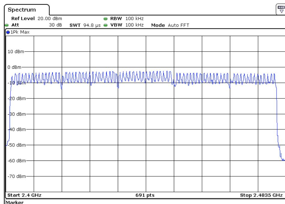
**Test result: The unit does meet the FCC requirements.**
