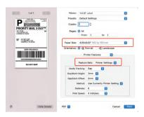
2.Click "Paper Size"->Choose the corresponding paper size according to the loaded label size. If the size you need is not listed, click "Manage Custom Sizes", input the width and height, then click "OK" (Please press button to calibrate before printing if you change loaded labels to another size.)
