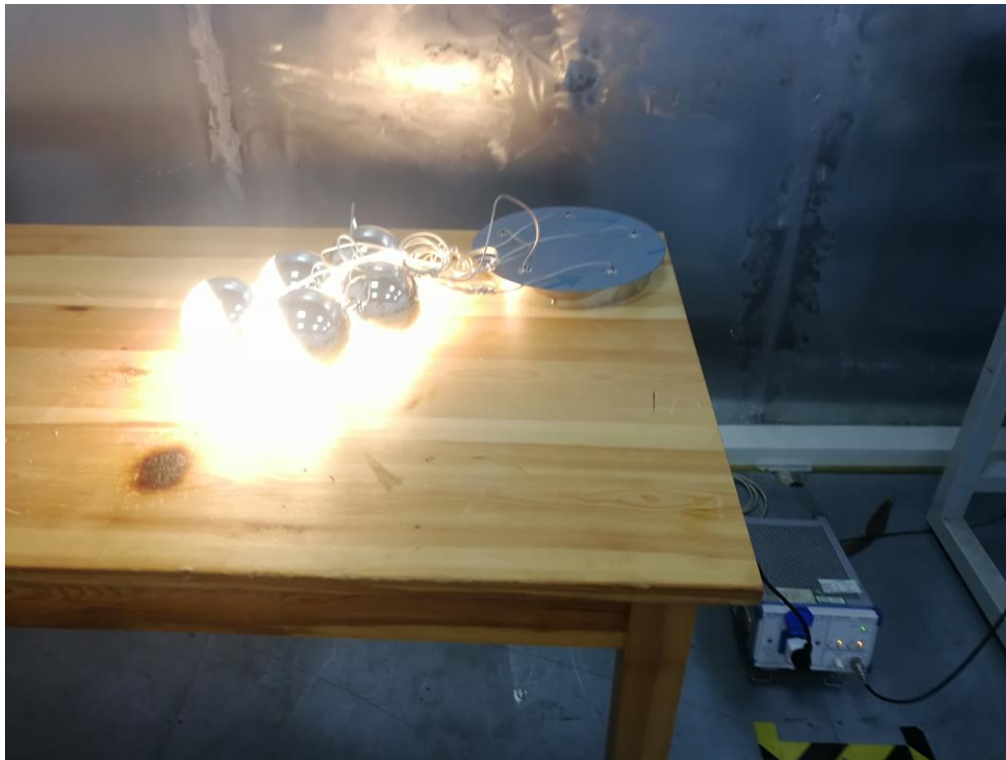
Photo of Power Line Conducted Measurement
