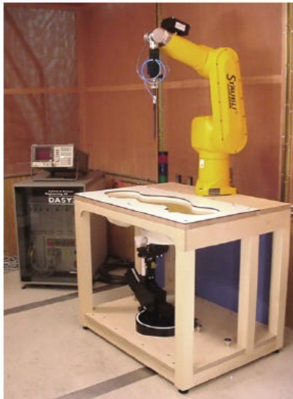
DASY3 SAR Measurement System with SAM Phantom
