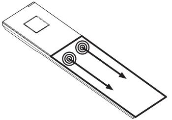
3. Lift the battery cover off the handset.
