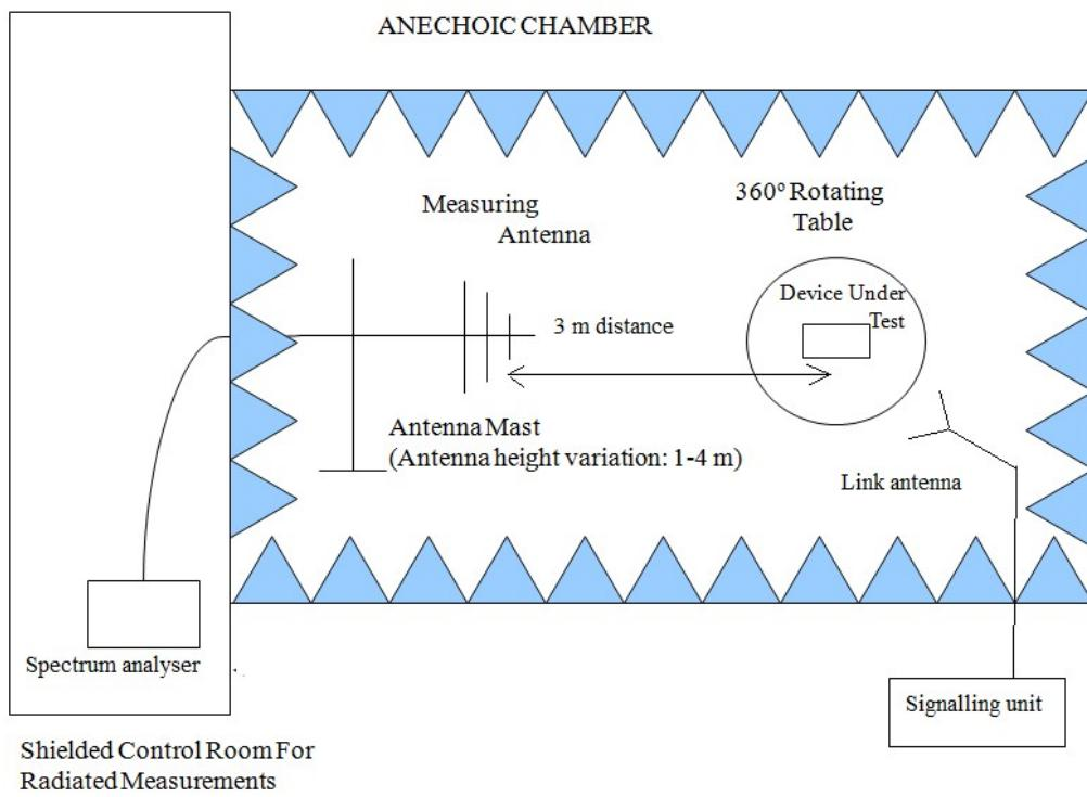
Radiated measurements above 1 GHz up to 18 GHz:
