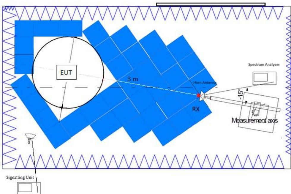
Radiated measurements above 18 GHz:
