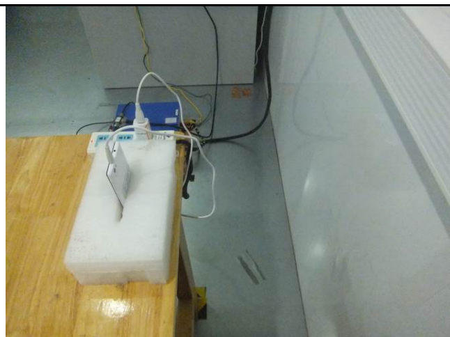
Conducted Emissions Test Setup Side View
