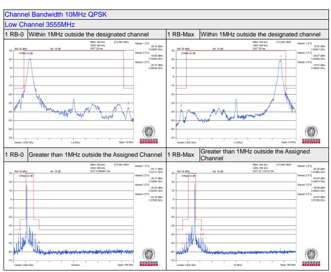
1MHz outside of designated channel needs to reduce the limit, When measured RBW less than 1MHz. Within 1- B MHz above the Assigned channel Limit is -13+10\*Log(100kHz/1MHz) = -23 dBm Within 1- B MHz below the Assigned channel Limit is -13+10\*Log(100kHz/1MHz) = -23 dBm B MHz above the Assigned channel Limit is -25+10\*Log(100kHz/1MHz) = -35 dBm B MHz below the Assigned channel Limit is -25+10\*Log(100kHz/1MHz) = -35 dBm
