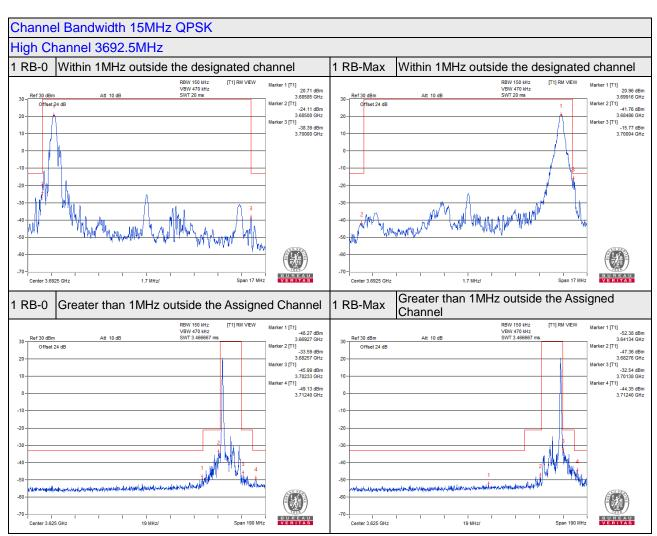
1MHz outside of designated channel needs to reduce the limit, When measured RBW less than 1MHz. Within 1- B MHz above the Assigned channel Limit is -13+10\*Log(150kHz/1MHz) = -21.24 dBm Within 1- B MHz below the Assigned channel Limit is -13+10\*Log(150kHz/1MHz) = -21.24 dBm B MHz above the Assigned channel Limit is -25+10\*Log(150kHz/1MHz) = -33.24 dBm B MHz below the Assigned channel Limit is -25+10\*Log(150kHz/1MHz) = -33.24 dBm
