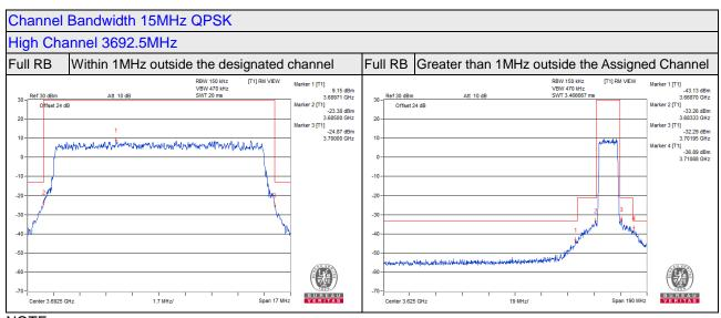
1MHz outside of designated channel needs to reduce the limit, When measured RBW less than 1MHz. Within 1- B MHz above the Assigned channel Limit is -13+10\*Log(150kHz/1MHz) = -21.24 dBm Within 1- B MHz below the Assigned channel Limit is -13+10\*Log(150kHz/1MHz) = -21.24 dBm B MHz above the Assigned channel Limit is -25+10\*Log(150kHz/1MHz) = -33.24 dBm B MHz below the Assigned channel Limit is -25+10\*Log(150kHz/1MHz) = -33.24 dBm
