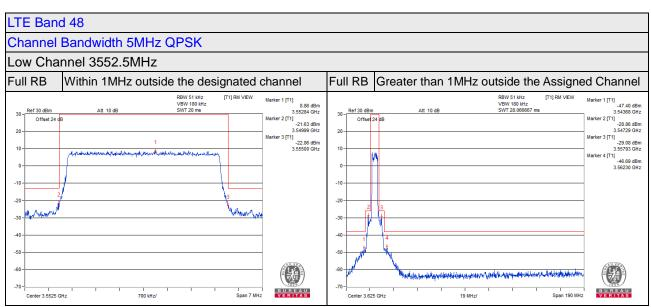
1MHz outside of designated channel needs to reduce the limit, When measured RBW less than 1MHz. Within 1- B MHz above the Assigned channel Limit is -13+10\*Log(51kHz/1MHz) = -25.92 dBm Within 1- B MHz below the Assigned channel Limit is -13+10\*Log(51kHz/1MHz) = -25.92 dBm B MHz above the Assigned channel Limit is -25+10\*Log(51kHz/1MHz) = -37.92 dBm B MHz below the Assigned channel Limit is -25+10\*Log(51kHz/1MHz) = -37.92 dBm
