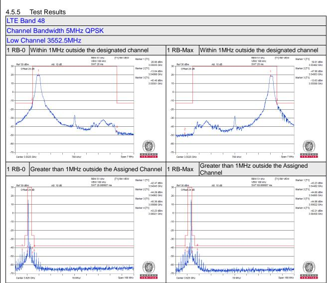
1MHz outside of designated channel needs to reduce the limit, When measured RBW less than 1MHz. Within 1- B MHz above the Assigned channel Limit is -13+10\*Log(51kHz/1MHz) = -25.92 dBm Within 1- B MHz below the Assigned channel Limit is -13+10\*Log(51kHz/1MHz) = -25.92 dBm B MHz above the Assigned channel Limit is -25+10\*Log(51kHz/1MHz) = -37.92 dBm B MHz below the Assigned channel Limit is -25+10\*Log(51kHz/1MHz) = -37.92 dBm
