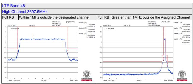
1MHz outside of designated channel needs to reduce the limit, When measured RBW less than 1MHz. Within 1- B MHz above the Assigned channel Limit is -13+10\*Log(51kHz/1MHz) = -25.92 dBm Within 1- B MHz below the Assigned channel Limit is -13+10\*Log(51kHz/1MHz) = -25.92 dBm B MHz above the Assigned channel Limit is -25+10\*Log(51kHz/1MHz) = -37.92 dBm B MHz below the Assigned channel Limit is -25+10\*Log(51kHz/1MHz) = -37.92 dBm
