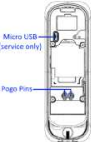
Doorbell Unit (inside view) —
