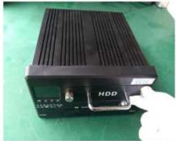
2. As shown in the figure, open the hard disk lock with the key, unscrew the fixing screw of the hard disk box, and pull out the hard disk.
