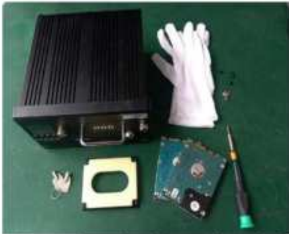
1. Prepare the tools and materials needed for installation: hard drive base, 2.5-inch hard disk, anti-static gloves, hard drive lock key, screwdriver, 8 M3*5 screws, 4 M3*6 screws
