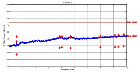
Final 1: 1.6 GHz, 50.0 kHz, 9.8 GHz; IF:1MHz, 100.0 ms MaxPeak, Att 0dB
