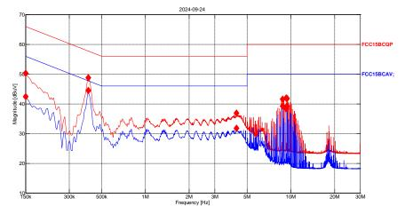
Scan1: 150.0 kHz, 5.0 kHz, 30.0 MHz; IF:9kHz, 15.0 s QP, Att AutodB, LISN-LISN\_2845\_Neutral-N
