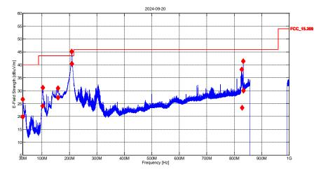
Final 1: 30.0 MHz, 50.0 kHz, 835.2 MHz; IF: 120 kHz, 200.0 ms QP, Att 10 dB
