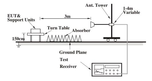
Note: For the actual test configuration, please refer to the Test Setup Photos exhibit.
