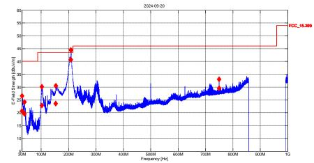
Final 1: 30.0 MHz, 50.0 kHz, 752.0 MHz; IF:120kHz, 200.0 ms QP, Att 10dB
