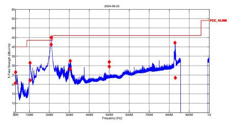
Final 1: 30.0 MHz, 50.0 kHz, 831.1 MHz; IF:120kHz, 200.0 ms QP, Att 10dB
