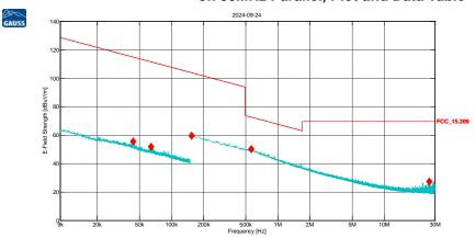
Scan1: 9.0 kHz, 100.0 Hz, 150.0 kHz; IF:200Hz, 100.0 ms MaxPeak, Att 10dB
