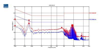
Scan1: 150.0 kHz, 5.0 kHz, 30.0 MHz; IF:9kHz, 15.0 s QP, Att Auto, LISN-LISN\_2845\_Line-L
