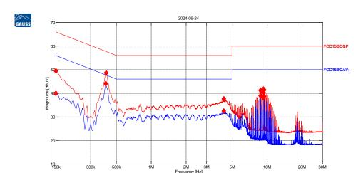
Scan1: 150.0 kHz, 5.0 kHz, 30.0 MHz; IF:9kHz, 15.0 s QP, Att Auto, LISN-LISN\_2845\_Line-L
