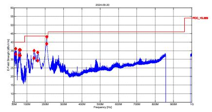
Final 1: 36.9 MHz, 50.0 kHz, 210.9 MHz; IF:120kHz, 200.0 ms QP, Att 10dB
