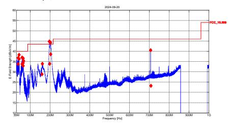
Final 1: 37.4 MHz, 50.0 kHz, 708.6 MHz; IF:120kHz, 200.0 ms QP, Att 10dB
