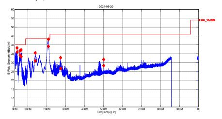
Final 1: 40.9 MHz, 50.0 kHz, 502.0 MHz; IF:120kHz, 200.0 ms QP, Att 10dB
