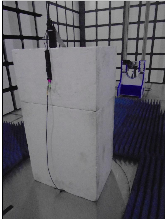
Figure 45 - Test Setup - 1 GHz to 2 GHz - Y Orientation
