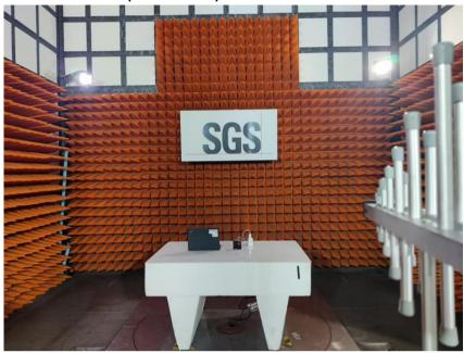
RF Radiated Test (Above 1GHz)
