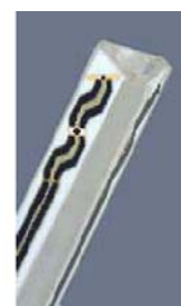
Figure 3.2 Probe Thick-Film Technique
