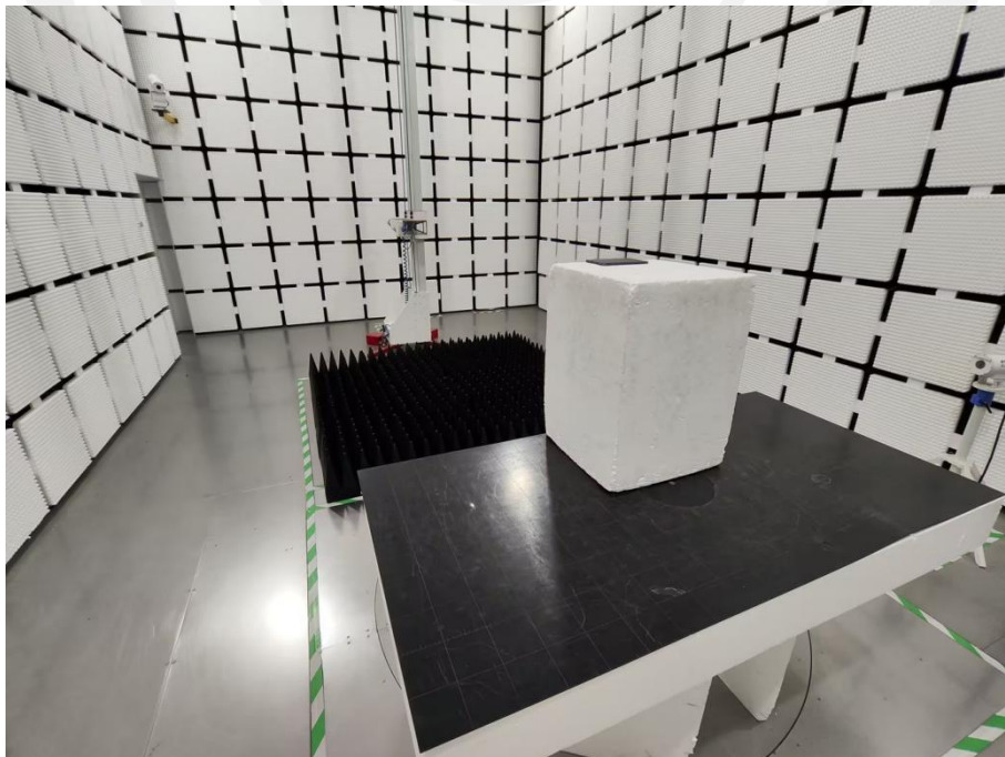
Spurious Radiation Emissions Test (> 1G)
