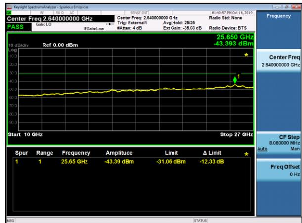
Spurious, 256QAM, 40MHz BW, 2610MHz, TX1
