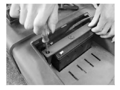
• Using a Phillips screwdriver, loosen the screws from the battery clamp. Remove the battery clamp from the battery compartment.
