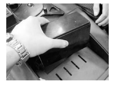
• Remove the 12 Volt (7.0 Amp/Hr.) battery from the battery compartment.
