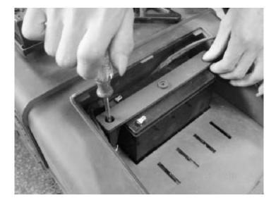
• Using a screwdriver, loosen the screws from the battery clamp. Remove the battery clamp from the battery compartment.
