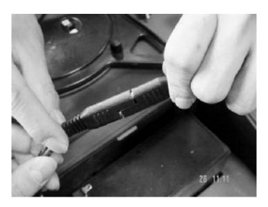
• Plug the battery connector into the HMMWV M1045A2 TOW Missile Carrier harness connector.
