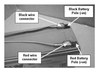
• **ATTENTION**: Make sure the battery connector wires are connected to the same color of the battery pole i.e. black color wire connected to the black color battery pole (-ve) and red color wire connected to the red color battery pole (+ve).
