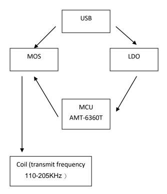
Working principle description: Supply power to the USB input, step down all the way to 5V through the LDO 7150 to supply power to the MCU master control, and the other to supply power to the MOS tube. After the main control is powered on, it outputs a PWM drive signal to drive the MOS tube, and the MOS tube drives the transmitting coil.
