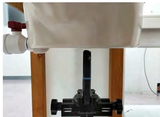
Fig.5 EUT Top side to flat phantom
