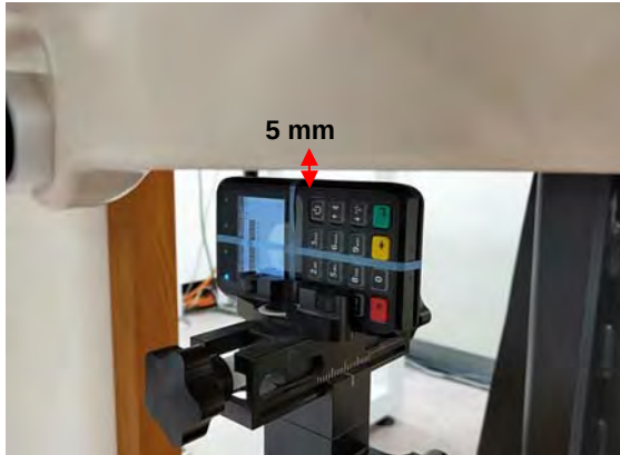
Fig.6 EUT Right side to flat phantom
