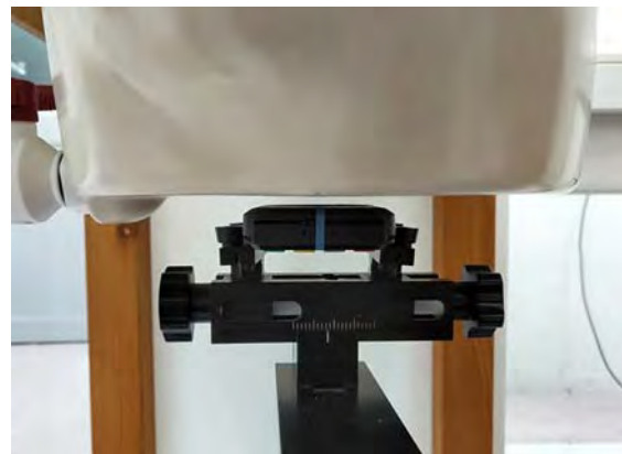
Fig.4 EUT Back side to flat phantom
