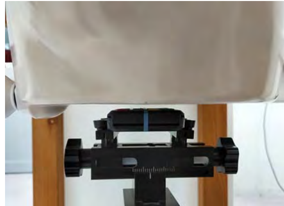
Fig.3 EUT Front side to flat phantom
