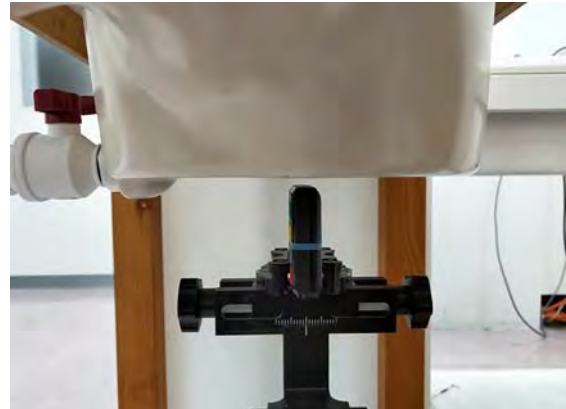
Fig.6 EUT Right side to flat phantom
