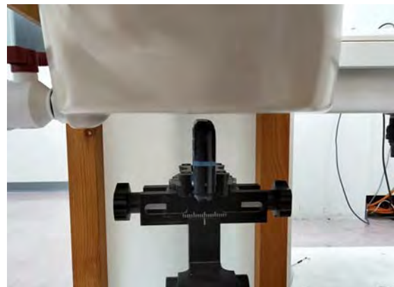
Fig.7 EUT Left side to flat phantom
