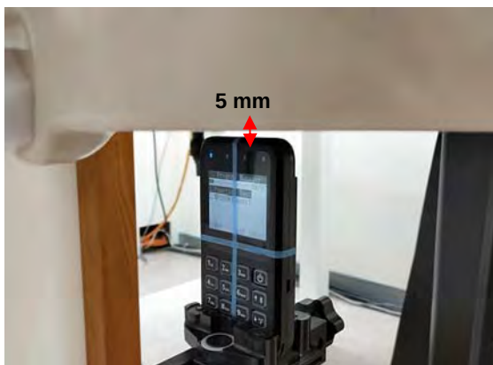
Fig.5 EUT Top side to flat phantom
