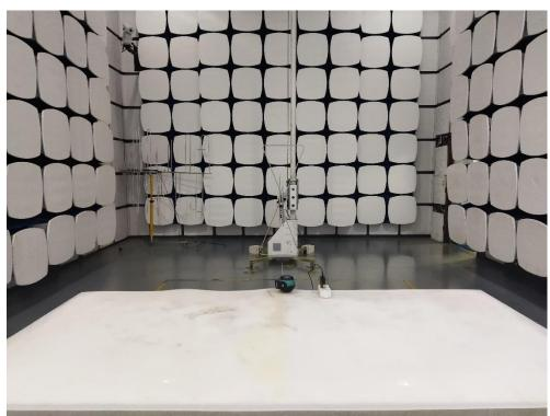
1.1. Photo of Radiated Emission test
