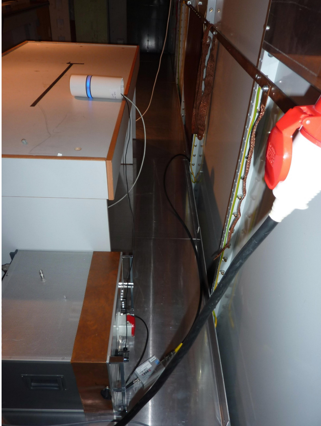
Test setup shielded chamber, EUT supplied via USB
