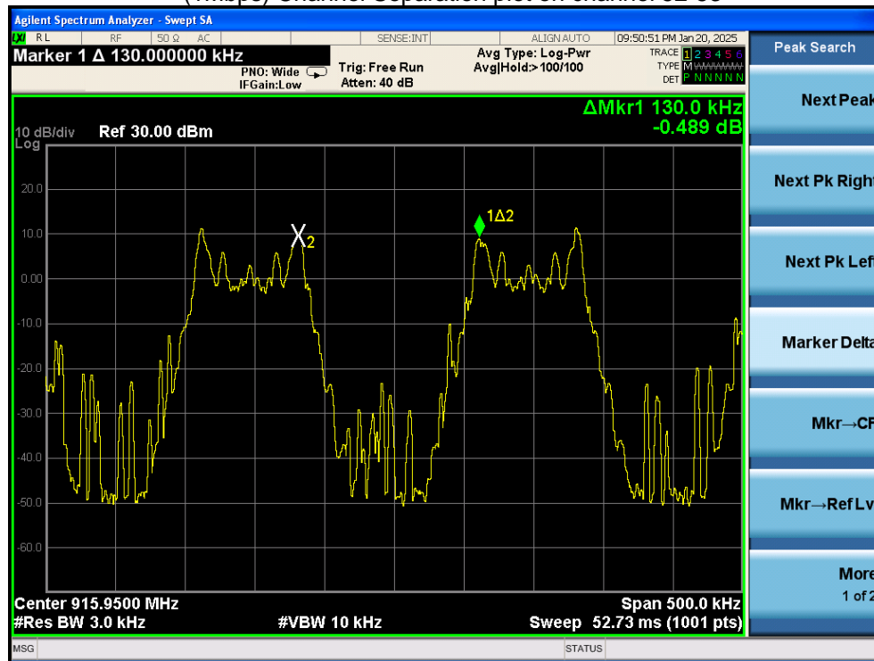
(1Mbps) Channel Separation plot on channel 102-103
