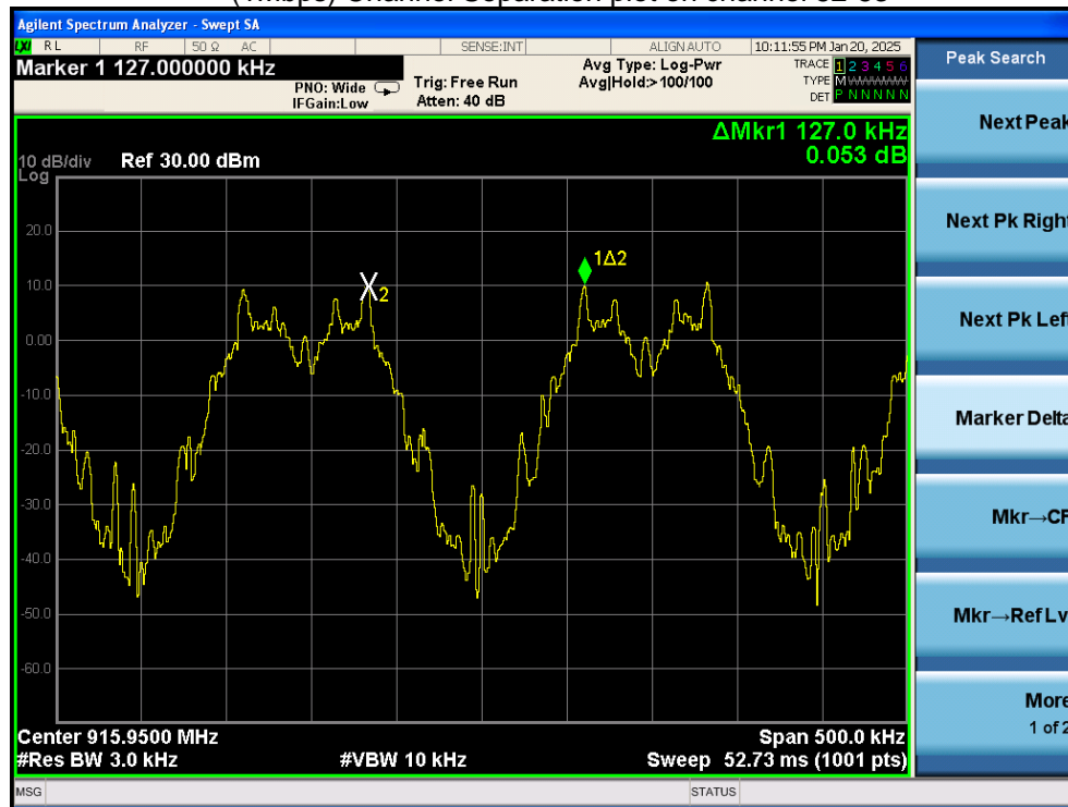
(1Mbps) Channel Separation plot on channel 102-103
