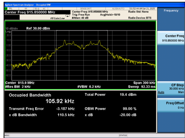
20dB Bandwidth plot on channel 52 (1Mbps)
