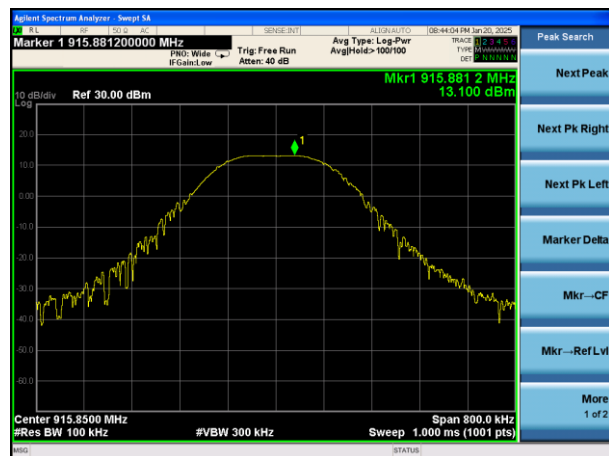
Peak output Power plot on channel 52 (1Mbps)
