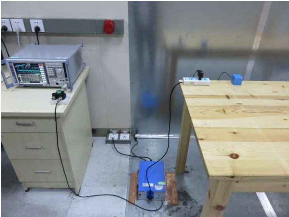
FCC RADIATED EMISSION TEST SETUP
