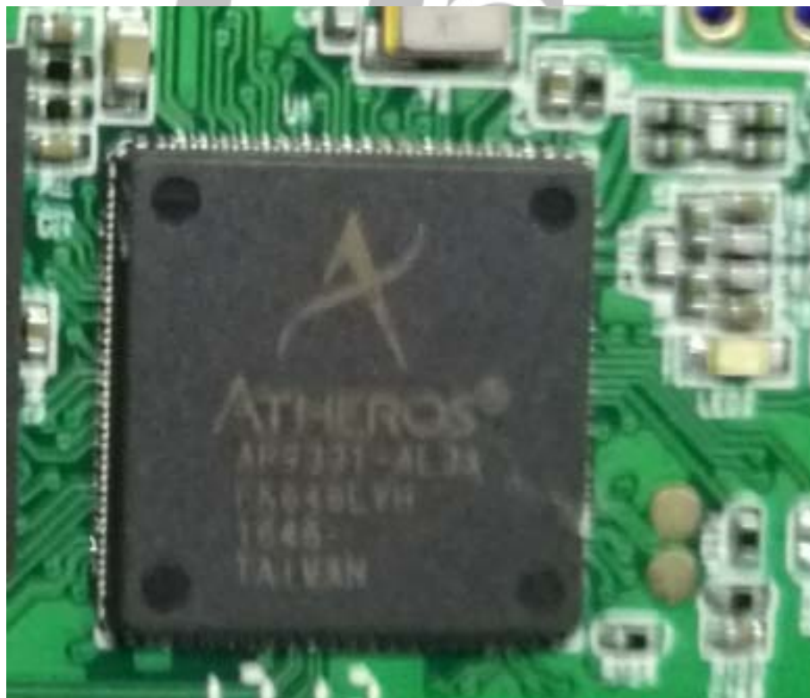
EUT –Wi-fi chip View
