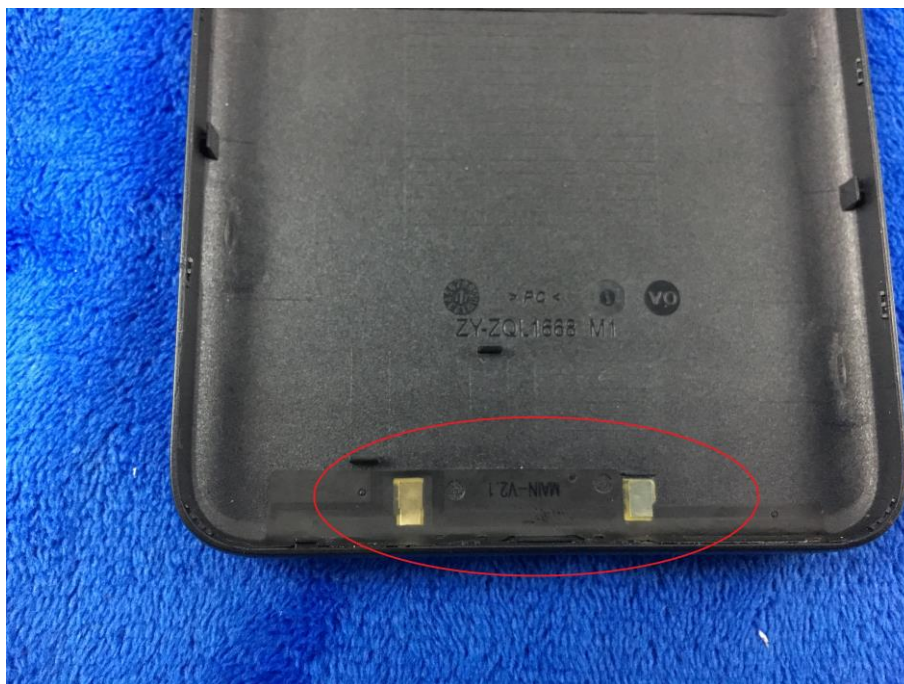
GSM/PCS/U MTS-FDD/LTE Antenna View
