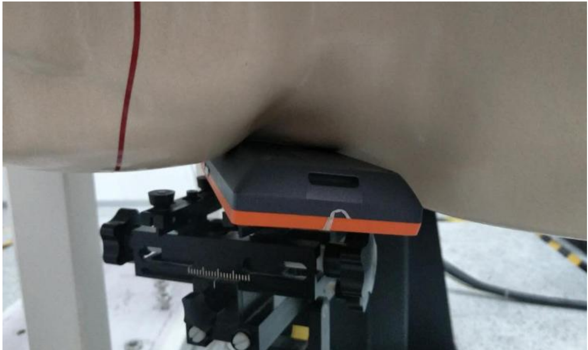
POSITION OF BODY BACK FOR WLAN WITH 0mm DISTANCE
