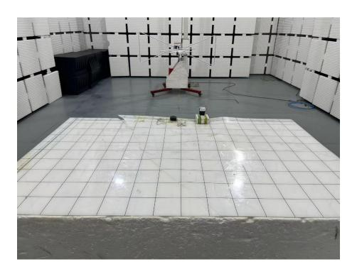
Set-up for Radiated Spurious Emission, Above 1GHz
