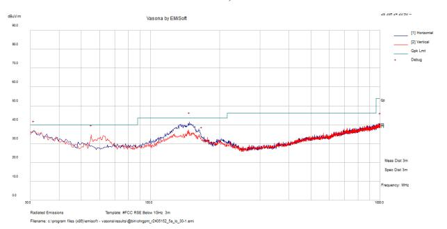
S.A. Correction Corrected Antenna **Antenna Turntable Frequency** Limit Margin Reading Factor Amplitude Height **Polarity Azimuth** Detector (MHz) (dBµV/m) (dB) (dBuV) (dB/m) $(dB\mu V/m)$ (cm) (H/V)(degrees) 147.37 49.47 -8.1741.3 300 Η 360 43.5 -2.2Peak 30.97 -1.65 36.84 300 40 38.49 Η 360 -3.16Peak 55.22 48.85 -14.2134.64 100 V 360 40 -5.36Peak 167.255 42.48 -8.82 33.66 300 Η 360 43.5 -9.84 Peak 1000 35.28 5.71 40.99 100 V 360 54 -13.01 Peak 46.92 -7.35 39.57 100 7 -3.93 135.982 Η 43.5 Peak
