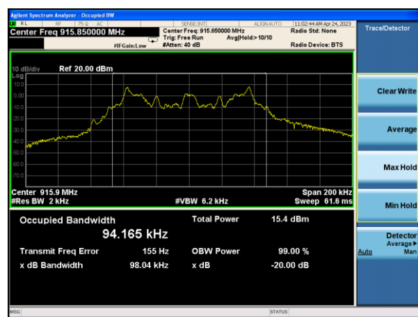
20dB Bandwidth plot on channel 52 (1Mbps)
