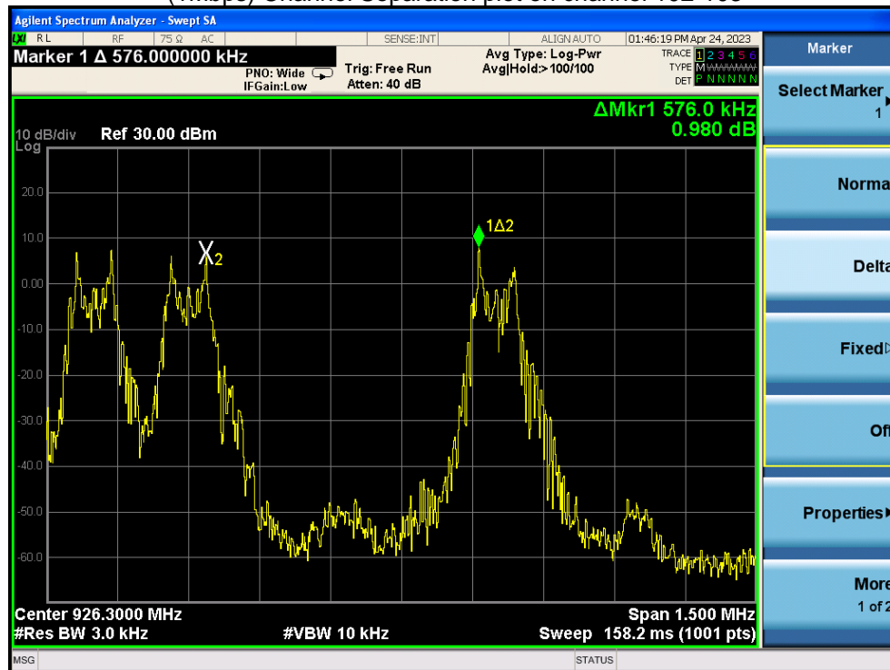
(1Mbps) Channel Separation plot on channel 102-103
