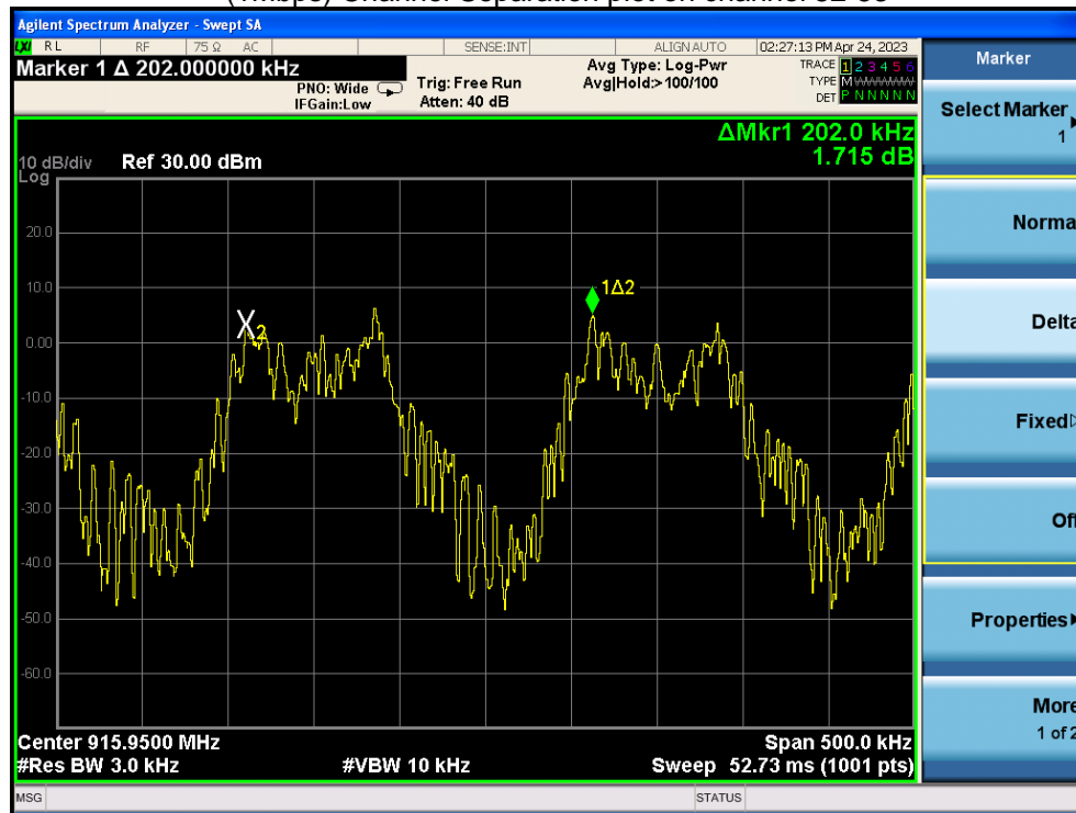
(1Mbps) Channel Separation plot on channel 102-103
