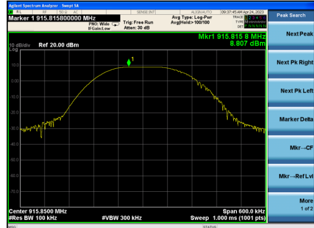
Peak output Power plot on channel 52 (1Mbps)
