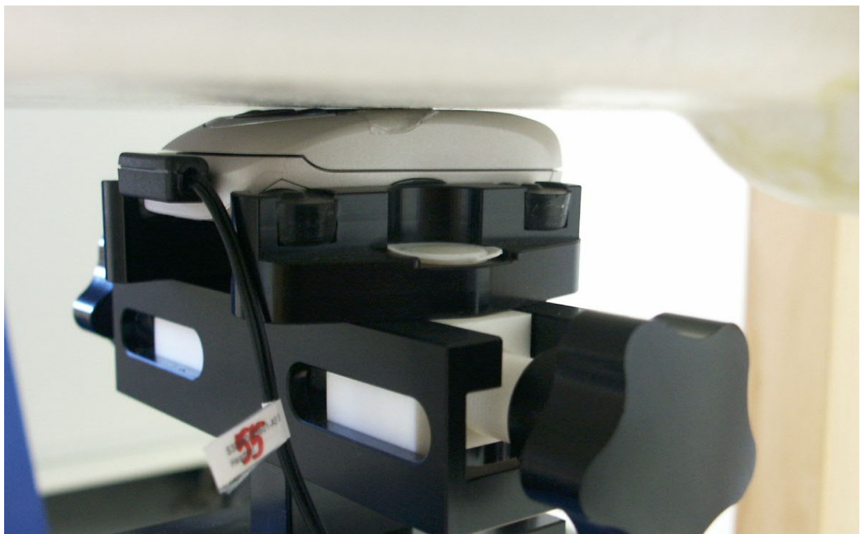
Fig. 45: Body worn configuration, slider down with headset, display towards the phantom.
