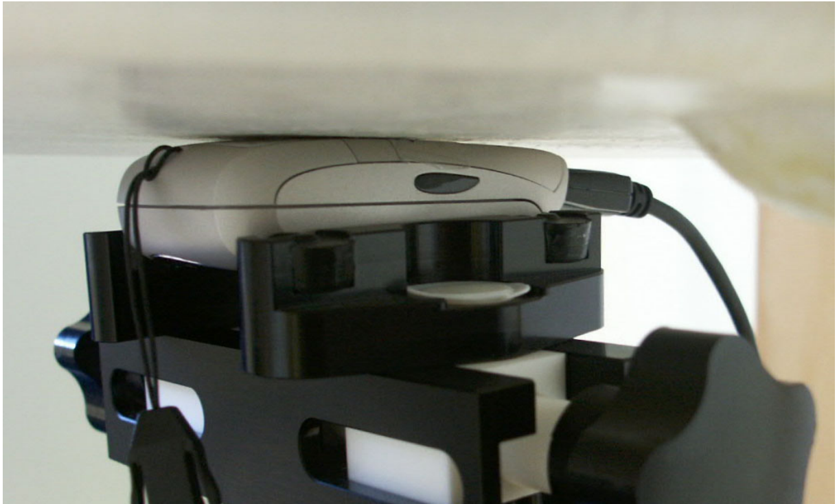
Fig. 46: Body worn configuration, slider down with data cable, display towards the ground.
