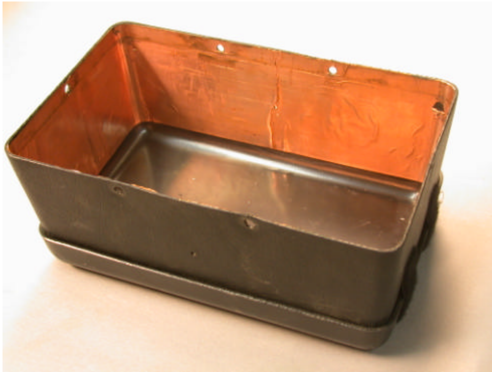
Picture 3. Plastic cover with EMC-shield.
