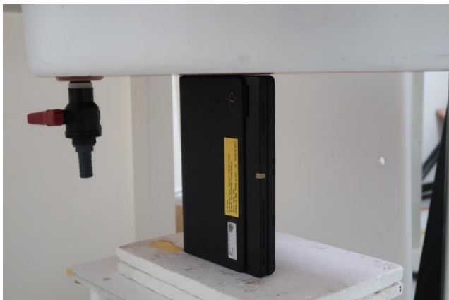
Right, Test Separation 0 mm
